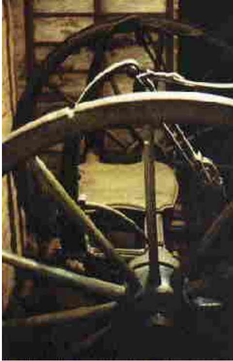
The rear F- or whip-springs of the Lister Chaise. - Photo: PG.
