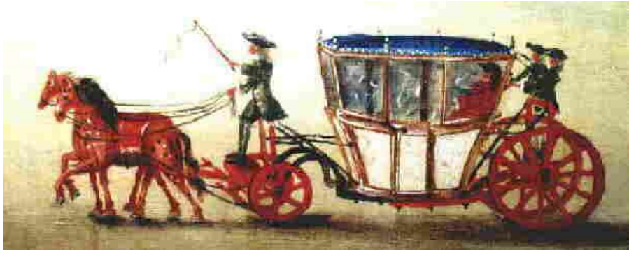
Germany, 1727: Berlin-undercarriage with iron crane-necks, suspension in the kind of the carosses (palace Weikersheim; photo: PG).
