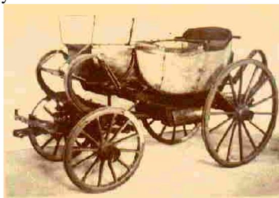
The military calash "de service leger" of Napoleon I, built by the (English?) coachmaker Getting (name engraved on the springs) in Paris, used during the campaign in 1805 and lost mysteriously after the battle of Austerlitz at the end of that year. The folding top is missing, the projection in front was for the legs when sleeping (cf Napoleon's equipages ). - Photo: Carriage Museum Wagenburg Schönbrunn, Vienna.
