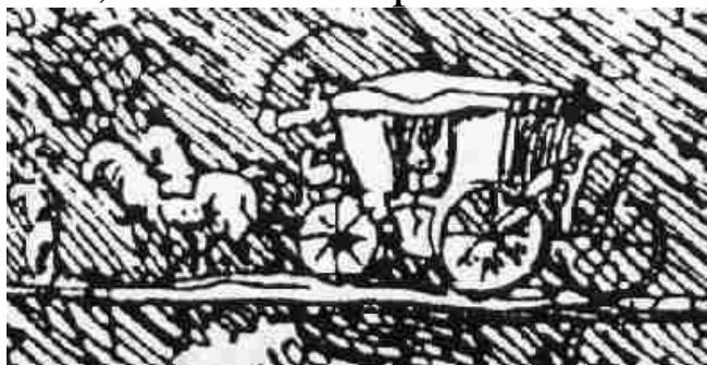
Presumably, the Carosse was an Italian invention, suspending the body between four supports. The undercarriage had - like always before - one perch. Left a design of a simple four-seater town and travelling carosse by Antonio Canal, about 1725. - Photo (cutting): PG. - - Another example of the same type. - From a painting by Giovanni Battista Tiepolo (1696-1770), or his school, in Orazio Bagnasco's palazzo in Venice (Ca' Contarini). Around 1740. Photo: PG.
